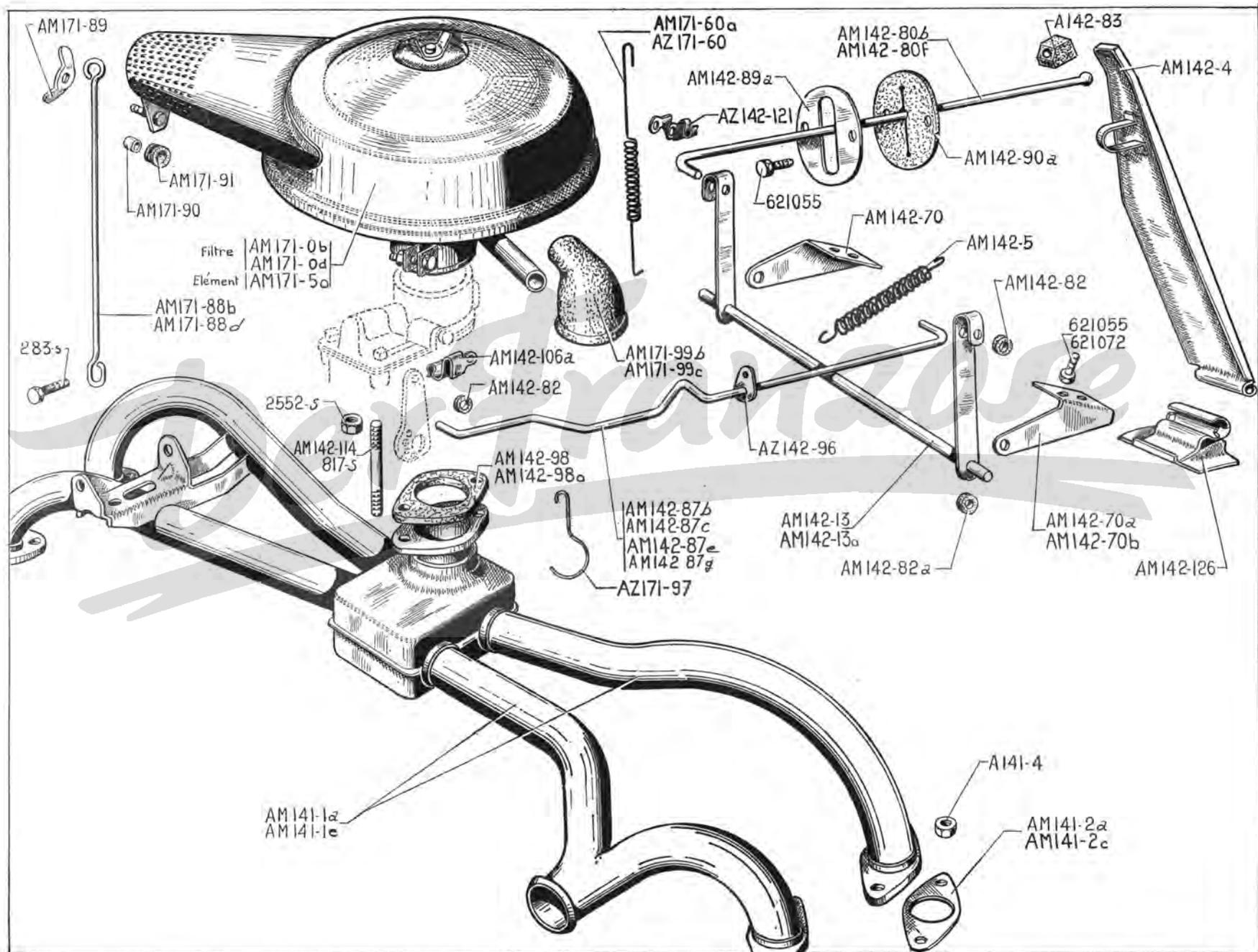
**CARBURATEUR ET SA COMMANDE - TUBULURE - FILTRE A AIR - DIRECTION A DROITE — 17**
