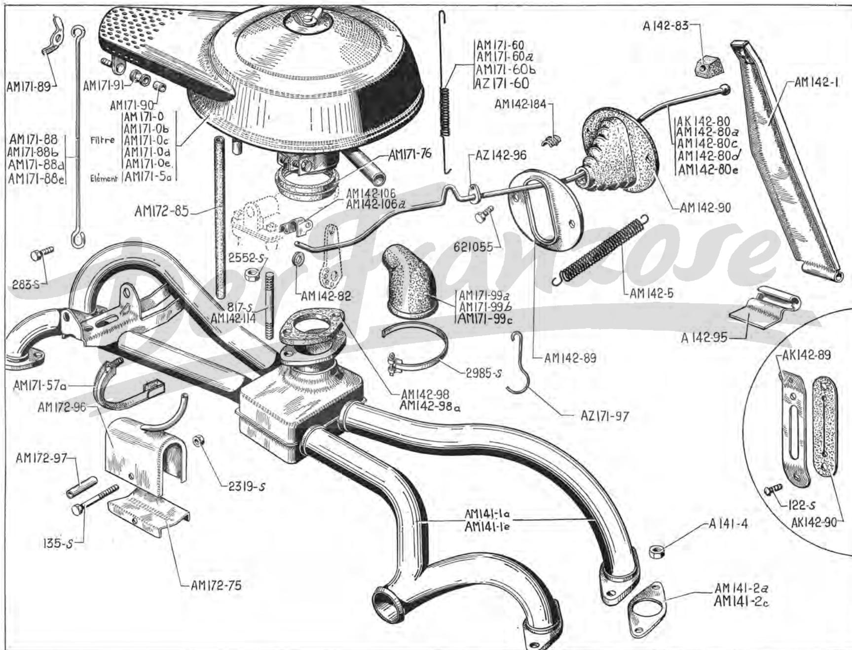
**CARBURATEUR ET SA COMMANDE - TUBULURE - FILTRE A AIR - DIRECTION A GAUCHE — 13**
